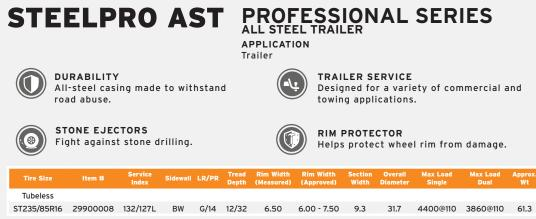
\*Trailer applications only. Requires special heavy-load capacity wheel. Consult wheel manufacturer for proper application
